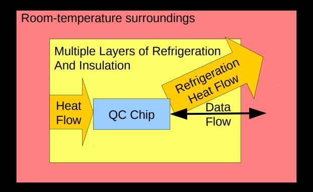
Heat is conducted along wires, and use of light for data delivers energy Liquid surroundings transport heat via convection Vacuum chambers transport heat via radiation Initialization and readout of quantum state generates waste heat
