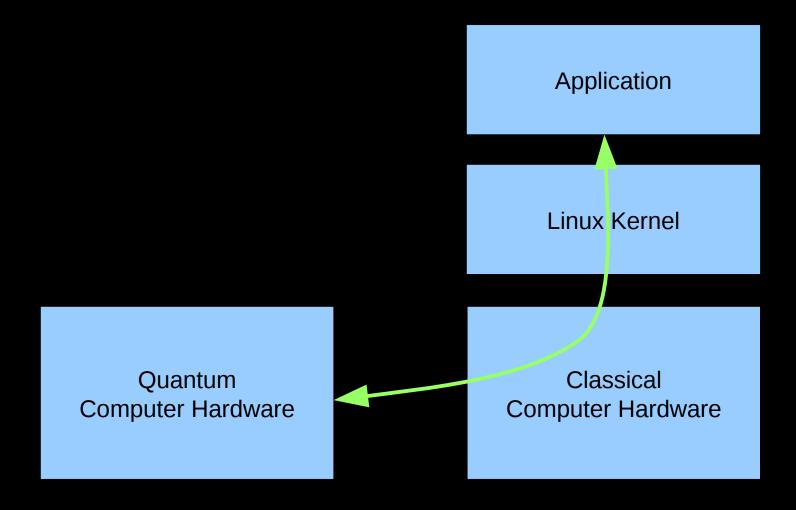
Accelerator, similar to GPGPU or FPGA
